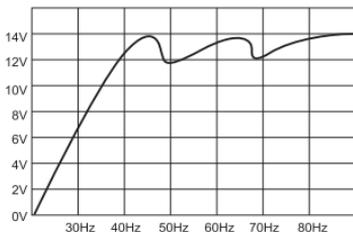
**Bassperformance at 50Hz and 70Hz with capacitor**
